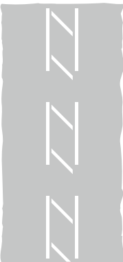
Diagonal white lines (hatched markings) bounded by broken lines may be used in the centre of the road to separate opposing flows of traffic. They are often provided at junctions to protect traffic turning right. They may also be used on the approach to a central traffic island or the start of a dual carriageway. Hatched markings with a single, broken boundary line may be used at the edge of the road or next to the central reservation of a dual carriageway: the diagonal lines always slope towards the direction of travel. You should not enter any hatched area bounded by a broken line unless it is safe to do so
