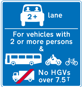
Another sign indicates which vehicles may use the HOV lane ahead
