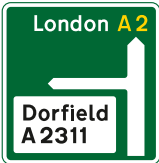
Sign on a primary route indicating a non-primary route
