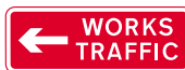
Sign to direct works traffic in advance of a road junction or works entrance
