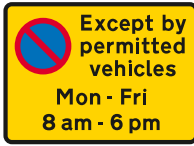
Repeater sign within a loading area
