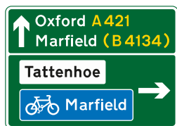
Primary route direction sign, in advance of a junction, indicating a route for cyclists
